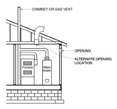
**Section 304.11 Combustion air ducts**
